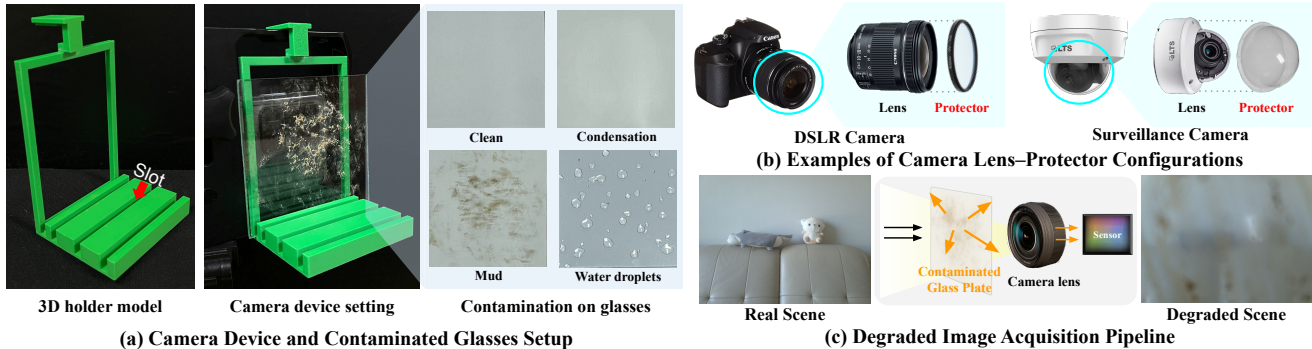
Figure 3. Data collection setup and devices equipped with lens protectors. (a) A custom 3D-printed smartphone holder designed to fix glass plates simulating contamination at fixed distances (0cm, 1cm, 3cm, 5cm). (b) Lens protectors are mounted at varying distances in different camera systems to protect the optics from contaminants. (c) By placing contaminated glass between the scene and the camera, our setup captures degraded images with realistic optical distortion and visual degradation.
